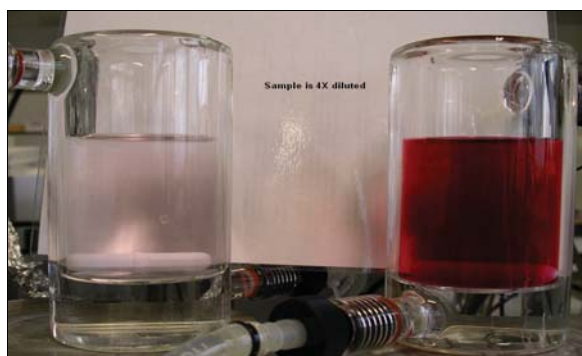
Waste water sample from dye house before (right) and after treatment with Dragon/Hydrogen peroxide (left)
